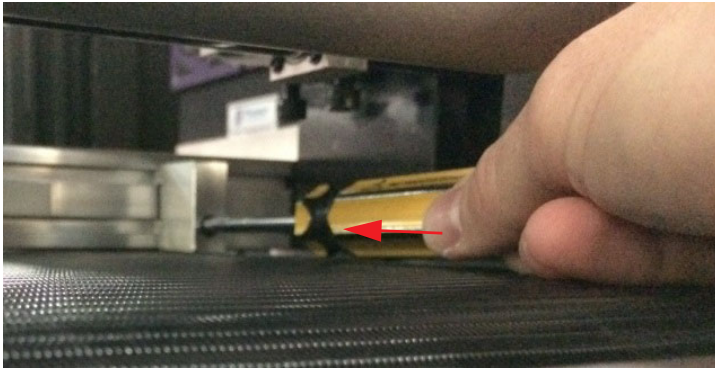
Figure 6-18: Loosen Screws on Guide Blocks
