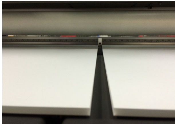
Figure 6-19: Press Each Board Against a Guide Block
