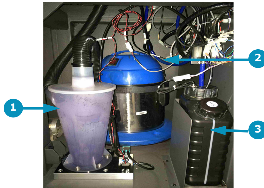
Figure 3-16: Waste Compartment (Cyclonic Vacuum System, Vacuum Canister and Ink Waste Container)
