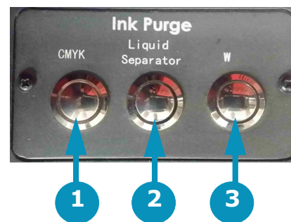
Figure 8-5: Manual Ink Purge Buttons (H1625 White Ink Printer Image Shown)
