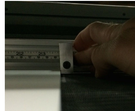
Figure 6-18: Place Guide Blocks Against Boards
