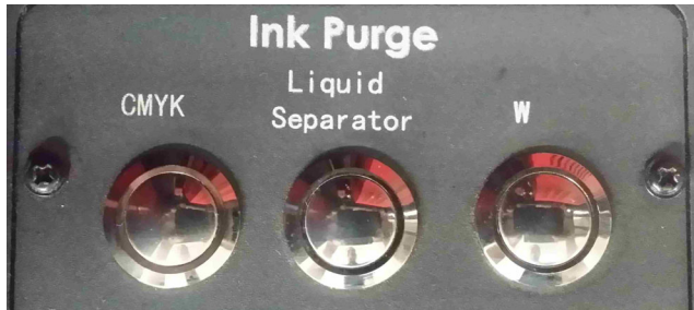
Figure 3-17: Liquid Separator -Empties Cyclonic Container
