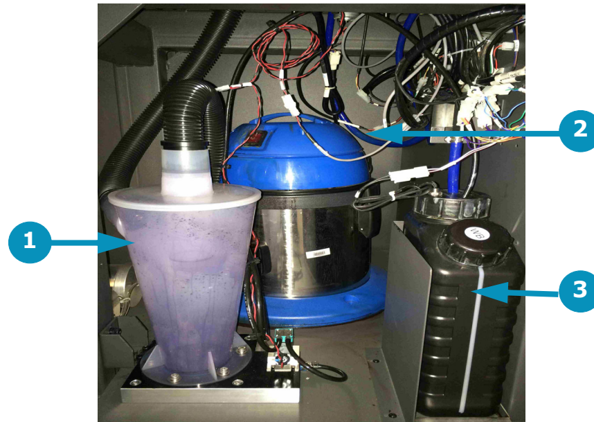
Figure 3-14: Waste Compartment (Cyclonic Vacuum System, Vacuum Canister and Ink Waste Container)
