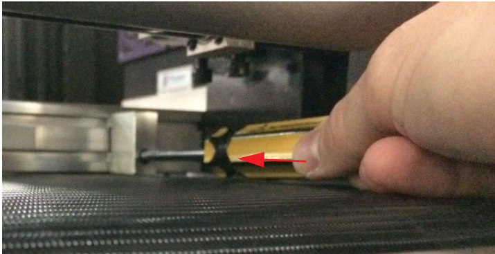
Figure 6-20: Loosen Screws on Guide Blocks
