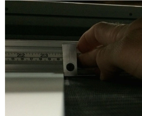
Figure 6-21: Place Guide Blocks Against Boards
