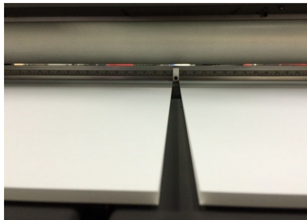
Figure 6-22: Press Each Board Against a Guide Block
