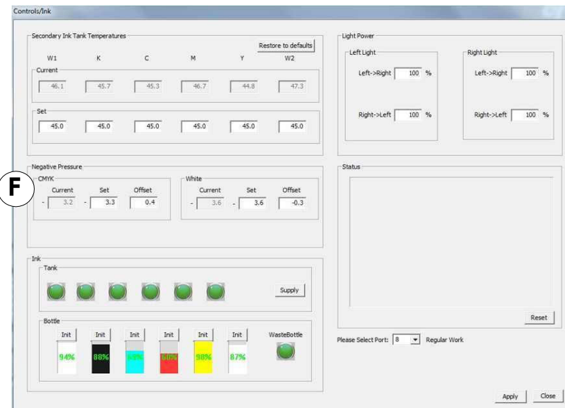
Figure 5-9 : PLC GUI (Controls/Ink Window)
