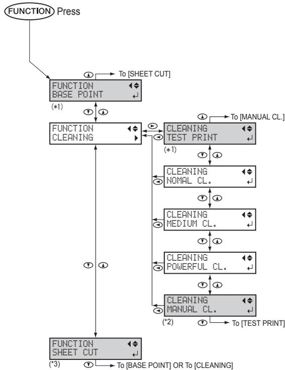
(\*1) This is not displayed when no media is loaded (that is, when **SETUP** is dark) or when the machine is not ready to set the base point. Refer to P. 42 "Setting the Printing-start Location" for details.
