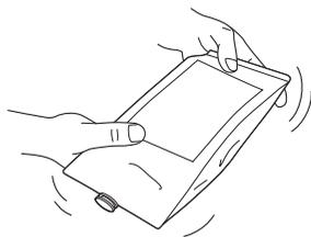
If ink components precipitate in the ink pouch, colors may be uneven (unevenness in printed colors). If colors are uneven, first remove the ink pouches, and shake them gently.
