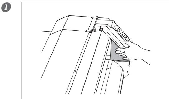
Touch the location shown in the figure to discharge any static electricity.
