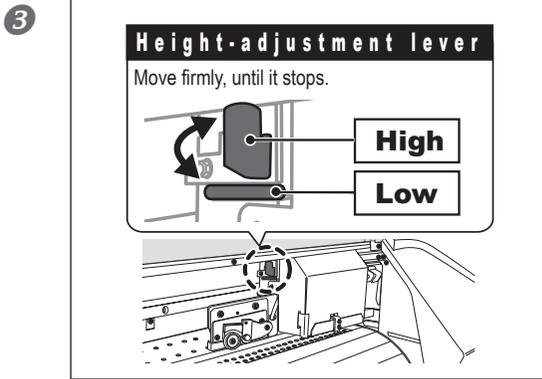
3 Move the height-adjustment lever to adjust the head height.
