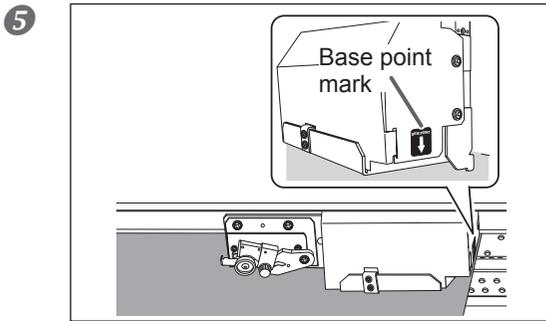
Press and to move the print-head carriage (base point mark) to the right edge of the media.
