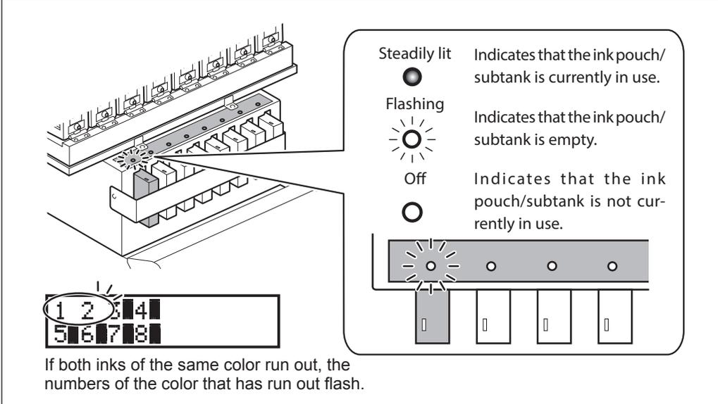
The diagram shows a top-down view of the ink pouches and a legend. The legend defines three states: 'Steadily lit' (solid circle) for 'currently in use', 'Flashing' (circle with radiating lines) for 'empty', and 'Off' (empty circle) for 'not currently in use'. Below the legend is a 2x4 grid of ink levels. The top row shows ink levels 1, 2, 3, and 4. The bottom row shows ink levels 5, 6, 7, and 8. In this example, ink levels 1 and 2 are flashing, while 3, 4, 5, 6, 7, and 8 are steadily lit.
