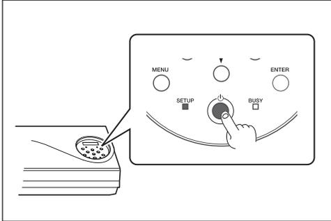
**Switch off the sub power whenever printing is finished.**
