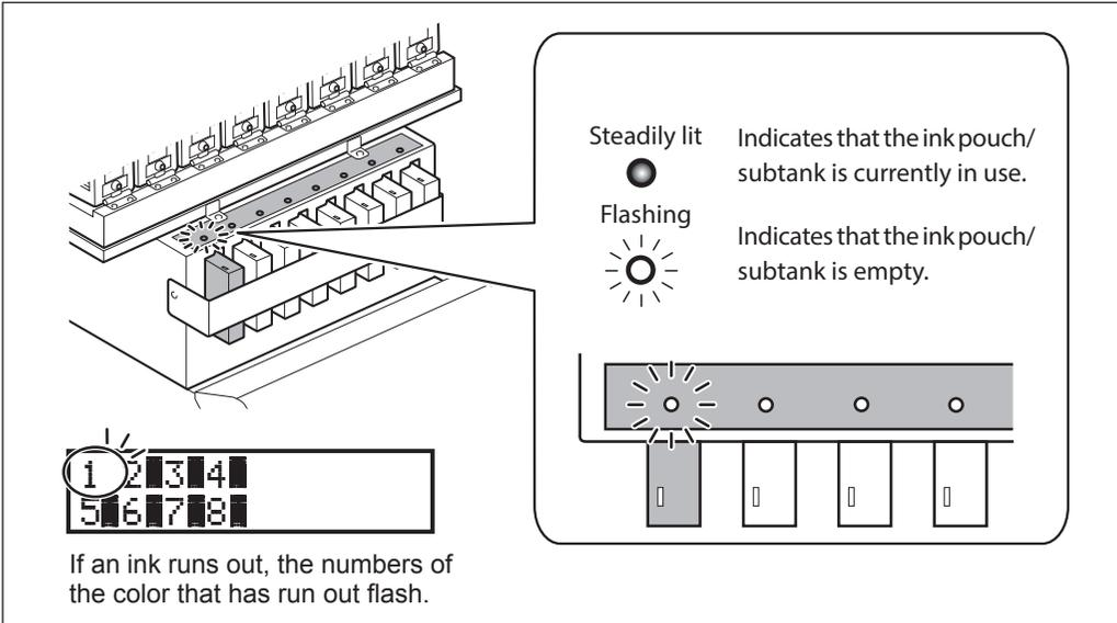
The diagram shows a top-down view of the ink pouches and a legend. The legend defines two states: 'Steadily lit' (solid circle) for 'currently in use' and 'Flashing' (circle with radiating lines) for 'empty'. Below the legend is a 2x4 grid of ink levels. The top row shows ink levels 1, 2, 3, and 4. The bottom row shows ink levels 5, 6, 7, and 8. In this example, ink level 1 is flashing, while 2, 3, 4, 5, 6, 7, and 8 are steadily lit.
