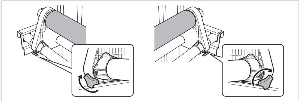
**2.** Pass the media through the machine and secure the media holders.
