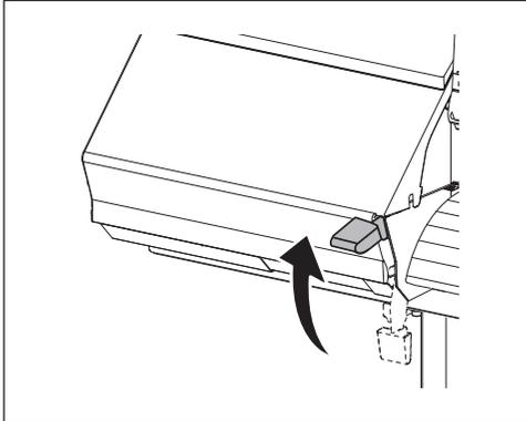
**Raise the loading lever and remove the media.**
