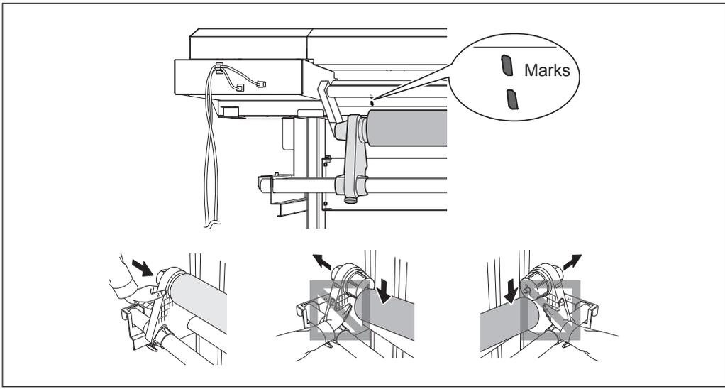
**IMPORTANT!** Decide the left and right side positions of the media finally at this step. After this procedure is completed, if the left and right side positions do not fit the proper position when securing the media with pinch rollers, go back to this step to redo this procedure. If you attempt to forcibly readjust the position of the media simply by pulling on the media itself, printing quality will be affected due to skewed media feed.
