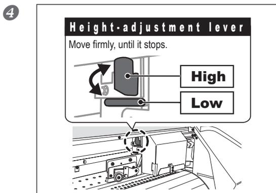
**Move the height-adjustment lever to adjust the head height.**
