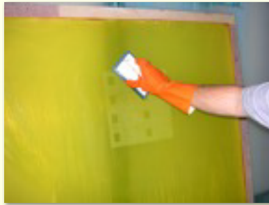
2. Scrub screen with non-abrasive pad or brush. Allow screen to dwell up to 10 minutes.
