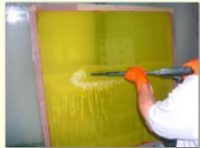
3. High pressure rinse - starting at bottom.
