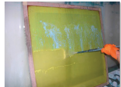
Step 3. High pressure rinse - starting at bottom.
