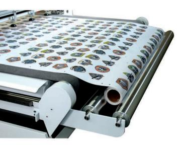
Incorporates an Automatic Roll Feeder for flexible media, making the length of the finished image virtually unlimited!
