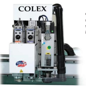
General purpose cutting and finishing system combining routing, knife cutting, creasing, perforating as well as textile cutting expanding your capabilities and dramatically increasing productivity. Ideal for shops with limited space.
