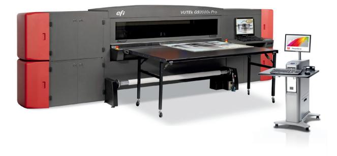
The 2-meter EFI<sup>™</sup> VUTEk<sup>®</sup> GS2000x Pro flatbed/roll-fed UV printer combines photorealistic print quality with high production speeds. It is ideal for replacing multiple lower productivity printers or can be added as a complementary piece of equipment to increase current printing capacity with a larger range of direct-to-substrate printing. Choose one of our thermoforming ink sets and transform your thermoforming business with direct-to-substrate printing.
