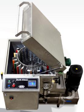
M&R's Qwik-Klean $^{\text{TM}}$  automates the highly labor-intensive, tedious process of cleaning squeegee holders and floodbars. Qwik-Klean achieves outstanding results through the combination of a high-volume spray and a rotating squeegee/floodbar holder assembly all within a single chamber. The addition of a final freshwater rinse eliminates the need for post-cycle washing and the possibility of squeegee degradation from chemical exposure.
