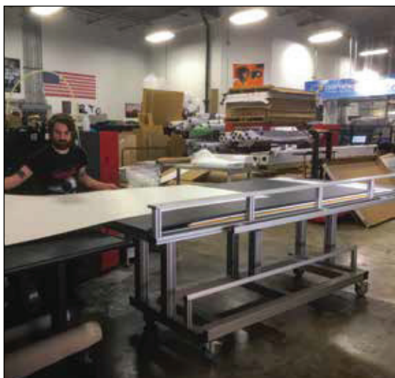
Operator can quickly and safely load boards onto printers and cutters.
