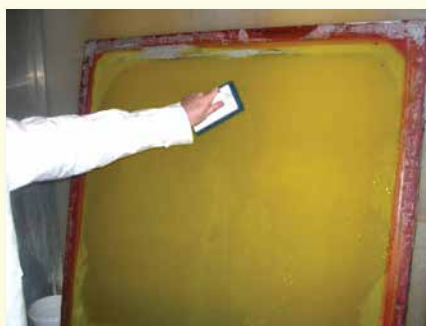
Step 2. Scrub screen with non-abrasive pad or brush.
