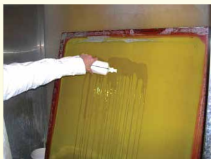
Step 1. After removal of ink, block-out, and emulsion, apply Prep-Rite to the screen(both sides).
