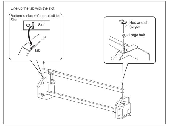
A Lay the unit on its side oriented as shown in the figure, then use large bolts to fasten the control box and the frame to the support bar.
