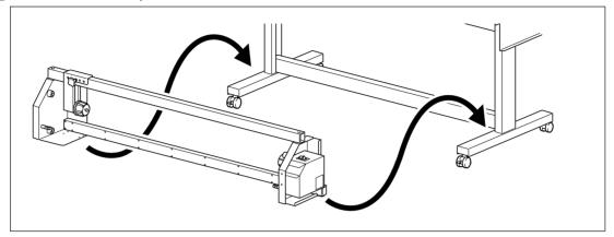
Obtermine where to secure the take-up unit in place.
