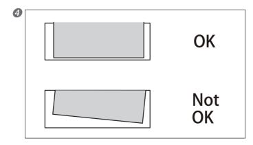
Load roll media onto the printer, then lower the loading lever. For information on how to perform loading, refer to the user's manual for the printer. After loading, check the following points.
