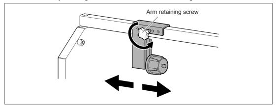
Attach the end caps to the paper tube and secure the arm in place. First, fit the paper tube securely onto the end cap on the same side as the right stand leg. Next, press the end cap on the same side as the arm into the paper tube and securely fit the end cap into the paper tube. Finally, secure the arm in place using the arm retaining screw.
