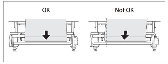
Using adhesive tape, fasten the center and side edges of the media to the paper tube (fasten a total of three locations).
