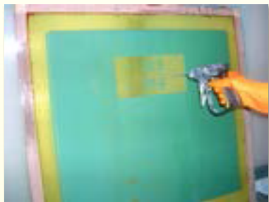
Step 1. After removal of ink, block-out, and tape, apply ER/80 to a wet screen(both sides).
