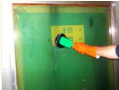
2. Scrub screen with non-abrasive pad or brush.
