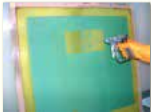
1) Card excess ink from screen, apply Microwash II to the screen (both sides).
