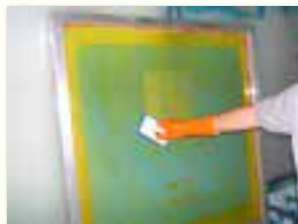
2. Scrub screen with non-abrasive pad or brush.
