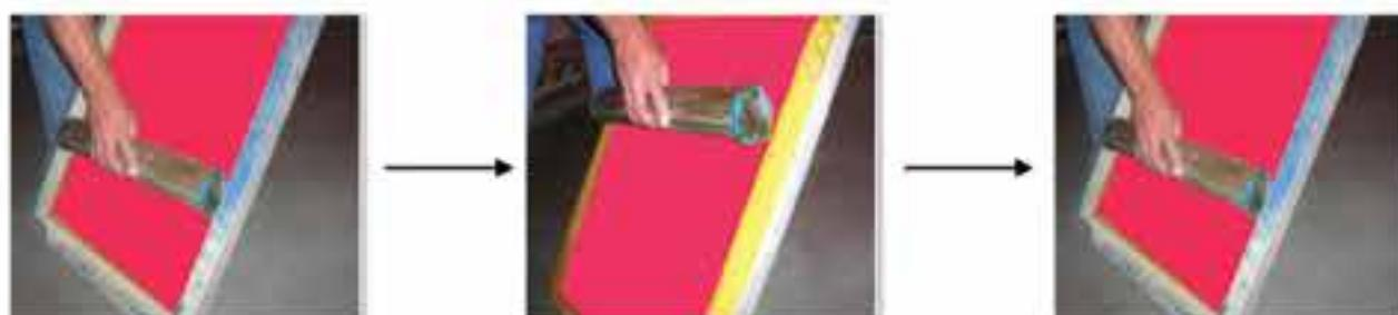
Slowly coat 4 times on the inside (that is the squeegee side), filling the mesh with emulsion. Then, in order to avoid air bubbles on the stencil, scrape the excess emulsion from the print side with another coater. This collected excess emulsion should be kept for subsequent use. After that, without drying, coat 6 to 18 times on the squeegee side, forcing the emulsion to the outside, creating thus a thick layer.
