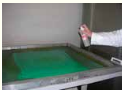
Step 1. Spray TS-305 on the squeegee side of screen.
