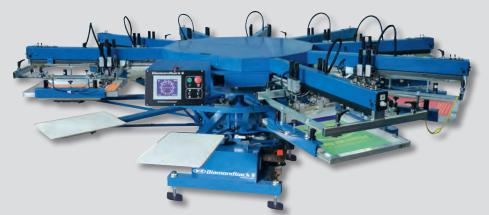
Diamondback S automatic screen printing press was the first press to bring servo drive to the entry-level user. It's available in 6, 7, 8 or 9 colors. It has a maximum image area of 41 x 46 cm (16" x 18"), and can accept screen frames up to 58 x 84 x 4.5 cm (23" x 33" x 1.75"). For those waiting for the right price on an entry-level automatic, the wait is over.
