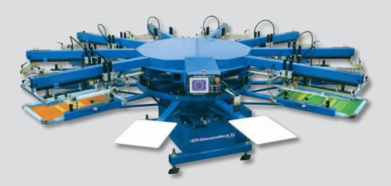
Diamondback XL automatic screen printing press combines servo drive, large image area, and affordability. Diamondback XL is available in 8 and 9 colors. It has a maximum image area of  $51 \times 53$  cm (20" x 21"), and can accept screen frames up to  $66 \times 91 \times 4.5$  cm (26" x 36" x 1.75"). It's the ideal press for large images at a low cost.
