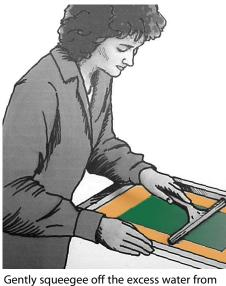
Spray the mesh, moving left to right and from the top to the bottom, and watch as capillary action draws the film's emulsion into the mesh. Be careful not to oversaturate the mesh. It doesn't take verv much water to apply the film.
