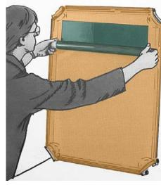
Roll the film down the wetted mesh. Use just enough pressure to ensure good contact of the emulsion to the mesh.
