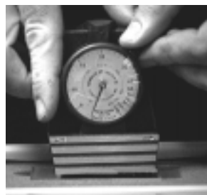
Incorrect alignment of needle to registration mark.
