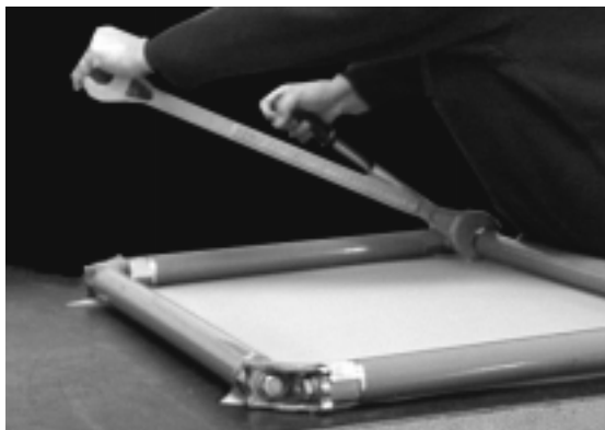
Applying downward pressure: corner flat.
