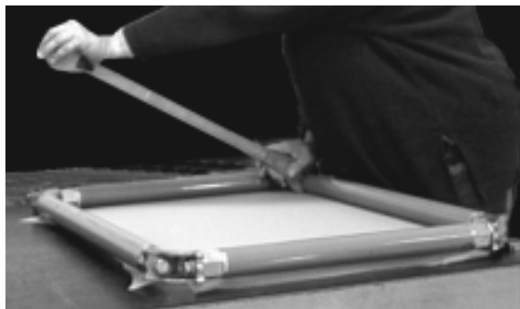
SDI wrench positioned at lowest possible angle.
