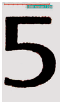
printed with SEFAR® LFM 150-32 (20x magnification)
