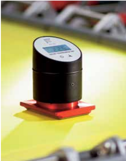
Checking the mesh tension with SEFAR® Tensotest 100: Equal high tension, less tension loss than conventional meshes
