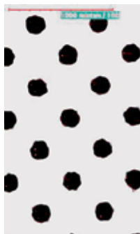
printed with SEFAR® LFM 150-32 (20x magnification)
