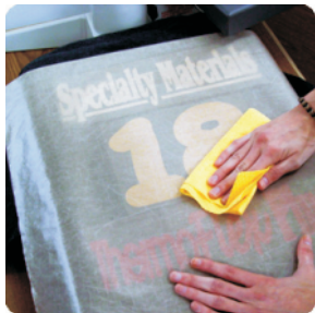
Rub design with pad or chalkboard eraser while still hot to dissipate heat
