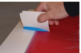
Apply Block-Out Spreads Block-out quickly and easily. Dispose of card when finished.
