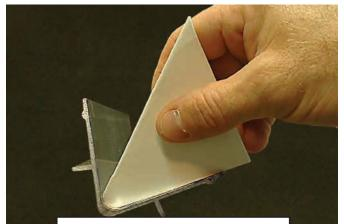
**Clean Scoop-coaters** Fold card diagonally in half to clean coaters. Saves time and expensive emulsion.
